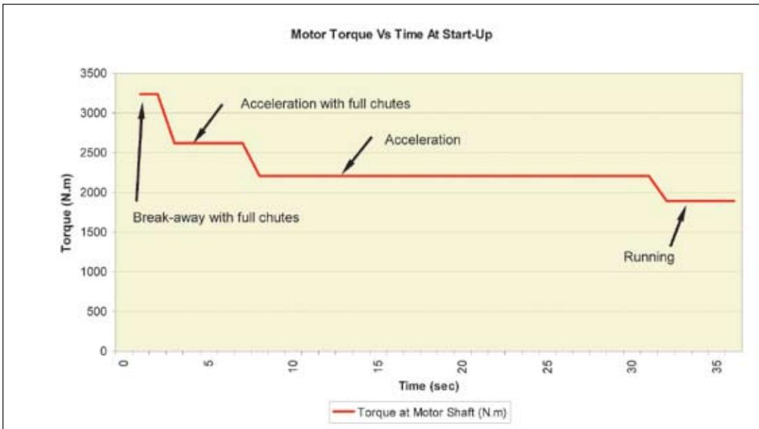
Figure 2. Example showing typical conveyor motor torque requirements during various phases at start-up.
