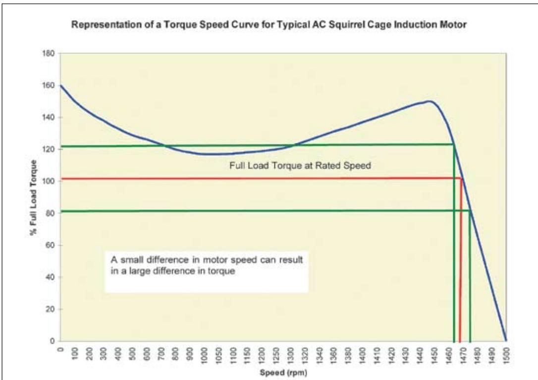
Figure 3. Representation of a typical torque speed curve for a squirrel cage induction motor.
