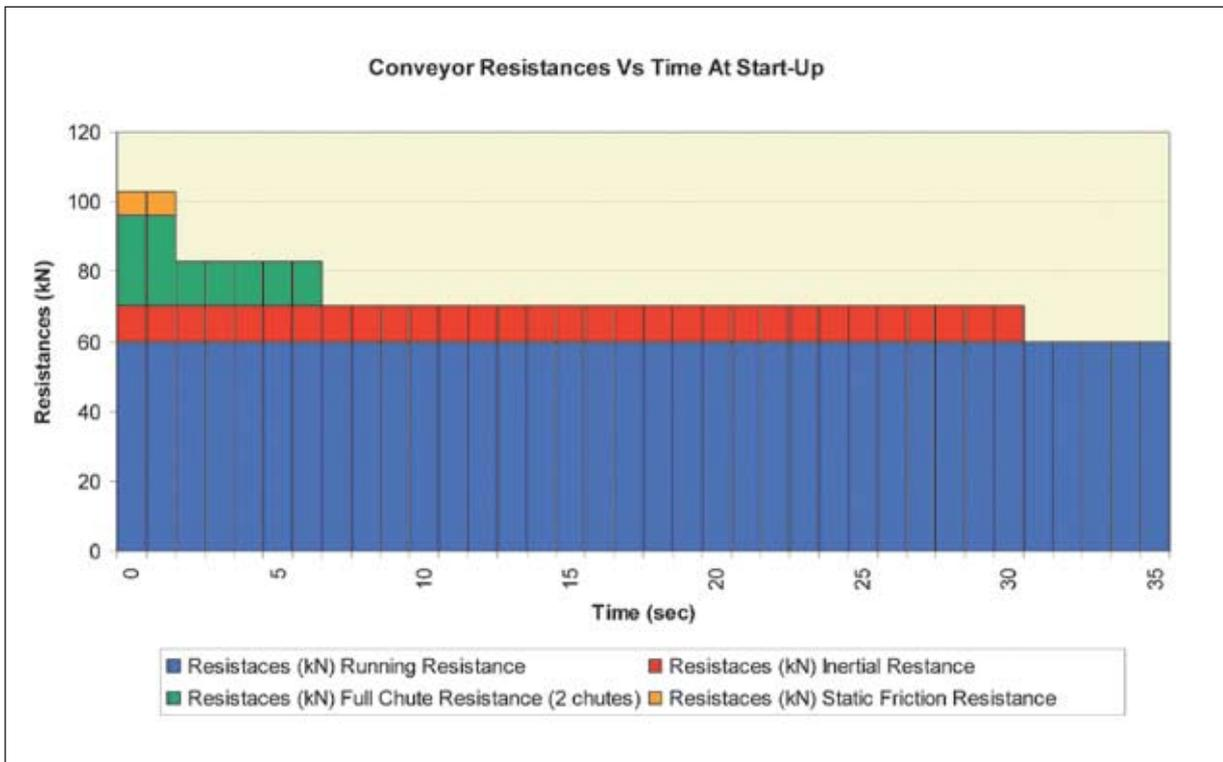
Figure 1. Example showing typical components of conveyor resistances at start-up.
